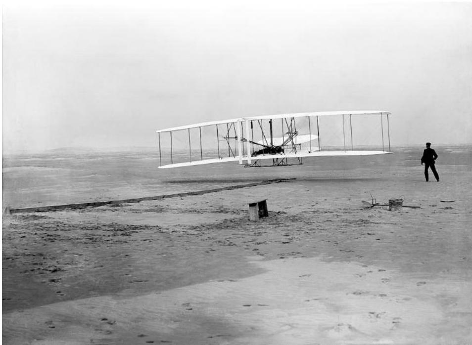
Helena Weiss was part of the acquisition of the Wright Flyer for the Smithsonian Institute. The Wright Flyer was the first powered, controlled, sustained airplane flight in history. Orville Wright, age 32, is at the controls of the machine, lying prone on the lower wing with hips in the cradle which operated the wing-warping mechanism. His brother, Wilbur Wright, age 36, ran alongside to help balance the machine, having just released his hold on the forward upright of the right wing. The starting rail, the wing-rest, a coil box, and other items needed for flight preparation are visible behind the machine. (Orville Wright preset the camera and had John T. Daniels squeeze the rubber bulb, tripping the shutter.)
